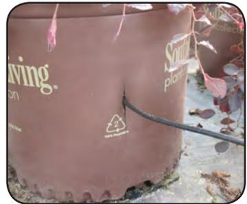
*Figure 39. Moisture sensors are placed directly into the container to measure substrate moisture level*
