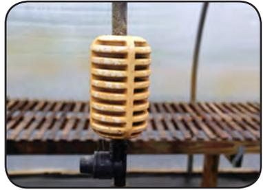
*Figure 16. Iron deposits can easily clog an irrigation or a mist system*
