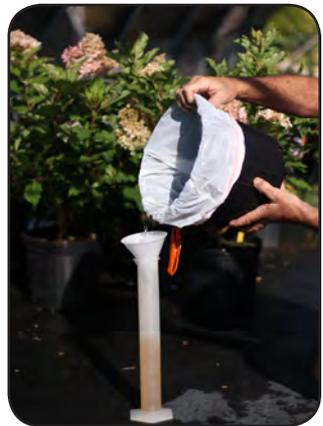
*Figure 58. Measure irrigation captured*
