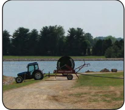
*Figure 29. Traveling guns are great for operations that do not need much irrigation*
