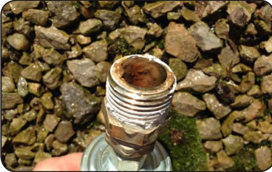
*Figure 17. Sediment in Irrigation lines*
