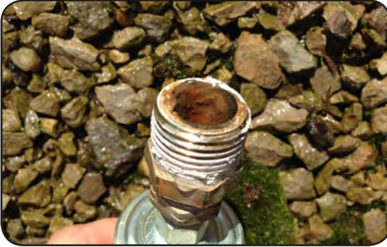
Figure 17. Sediment in Irrigation lines
