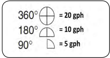
Figure 47. Selecting nozzles to provide matched precipitation
